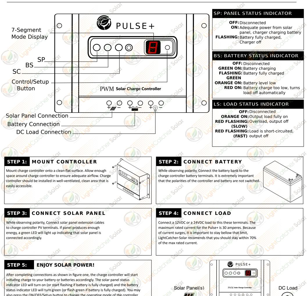
also press the ON/OFF/Setup button to change the operating mode of the controller to control the load output. For more on modes of operation, please refer to Mode Operation table below.
